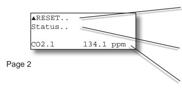
Press the ← key in this line to enter a submenu to reset the calibration parameters (■ 6.2.2.2.1, page 6-8)
